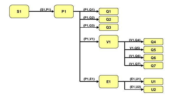
Figure 9. A Distributed Transaction Calling Hierarchy
