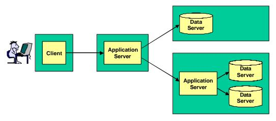
**Figure 6. A Common Distributed Application Architecture**
