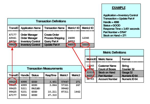
Figure 14. Combining Ids and Handles With Descriptive Information
