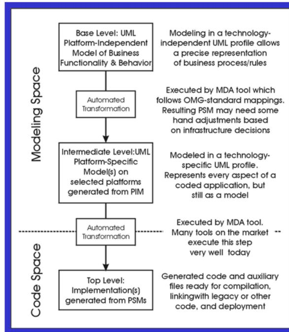
The next step is the transformation of the PIM to a PSM, using OMG standard profiles that extend UML to embrace the semantics of the target platform. As with the PIM, it is conceivable that levels of abstraction can occur here. For example, a PSM may reflect a generic component-based platform, which in turn could be further specialized to a CORBA Component Model or Enterprise Java Beans.
