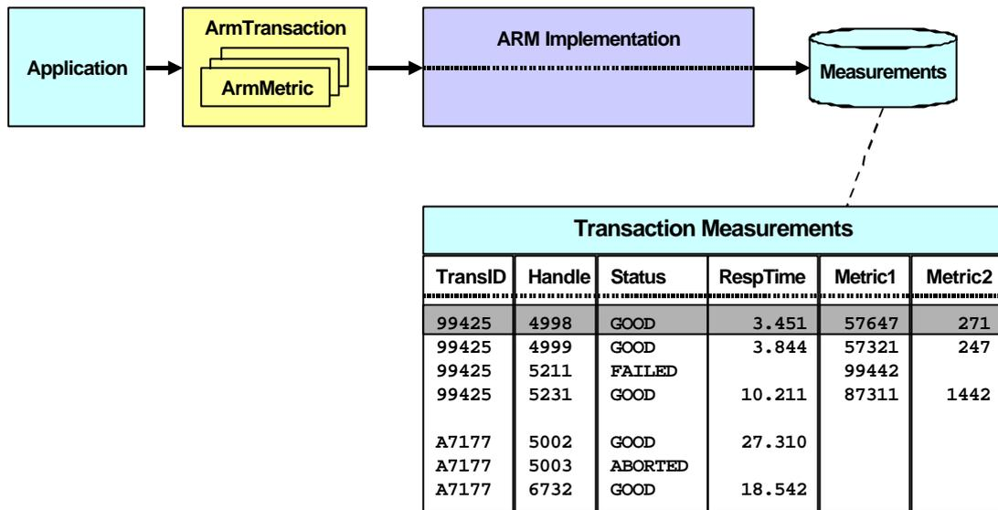
**Figure 13. Providing Measurements Without Any Descriptive Information**
