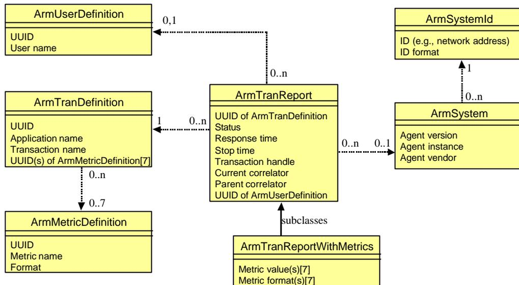
Figure 18. ARM 3.0 Data Model Using ArmTranReport
