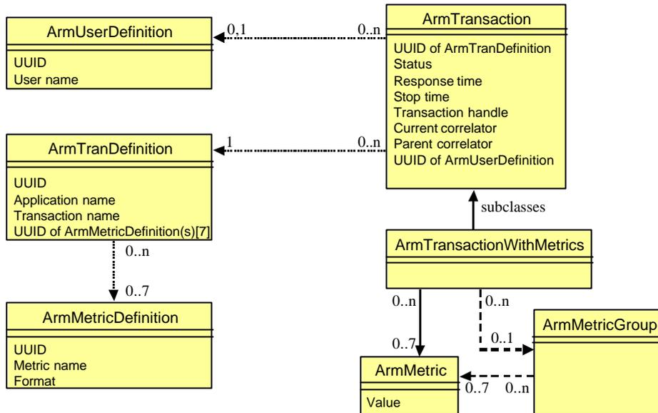
**Figure 17. ARM 3.0 Data Model Using ArmTransaction**
