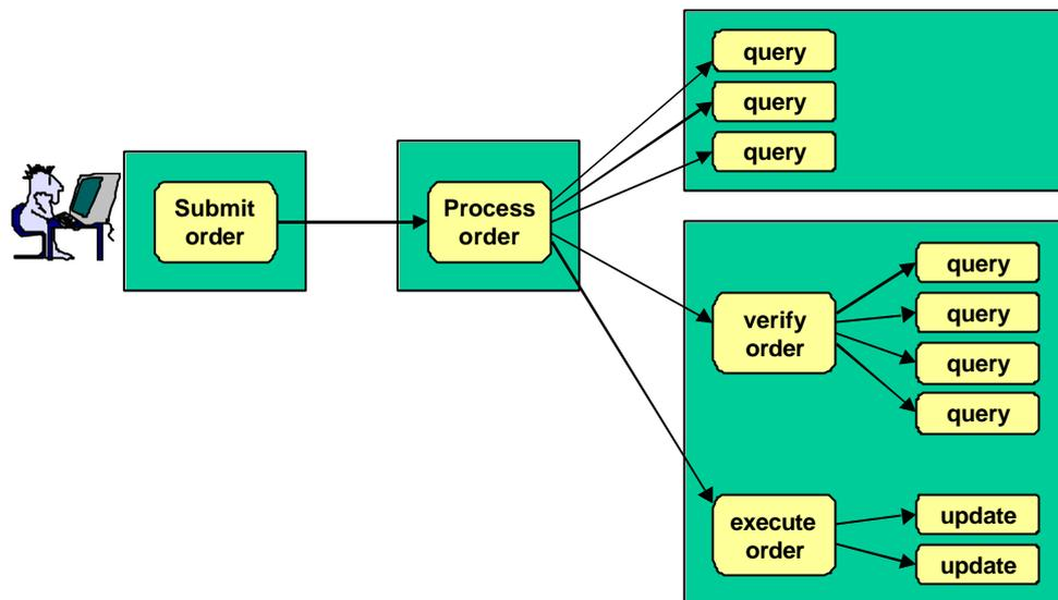
**Figure 7. An Example of a Distributed Transaction**
