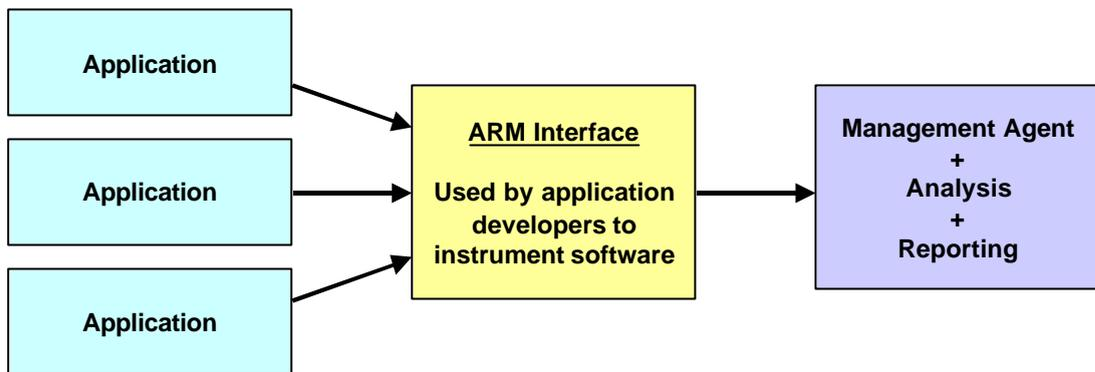
**Figure 2. Application - ARM - Management System Interaction**
