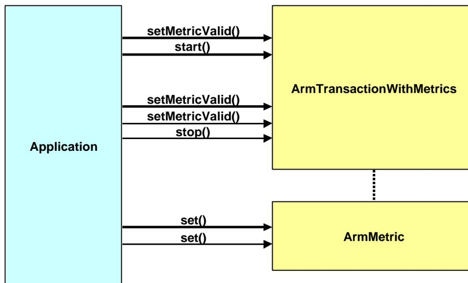
**Figure 10. Providing Additional Data Using ArmTransaction and ArmMetric**
